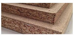
Particle board is the lightest board in fiber boards and with less strength to MDF board and other hard woods. Moreover, particle board will expand easily when exposed to the moistness. However, particle board is popular for interior usage as it has light weight, cheap and easy to move. In addition, particle board is environmental-friendly as no hard woods in the forest shall be cut down.
