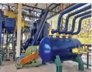
Gasification technology is the use of biomass fuel to burn in a specially designed furnace which is called as "Gasifier stove", it will control the amount of air entering the furnace in lesser volume than usual to force the situation which is called "Incomplete combustion". Such condition will cause the heat inside the stove approximately 1100 degrees Celsius and there are five types of gas occurred:
