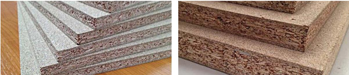
Particle board is the lightest board in fiber boards and with less strength to MDF board and other hard woods. Moreover, particle board will expand easily when exposed to the moistness. However, particle board is popular for interior usage as it has light weight, cheap and easy to move. In addition, particle board is environmental-friendly as no hard woods in the forest shall be cut down.
