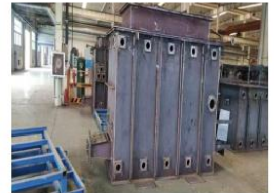
Inverter station Oil tank production
