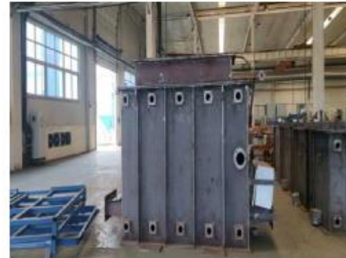
Inverter station Oil tank production
