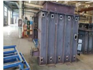
Inverter station Oil tank production
