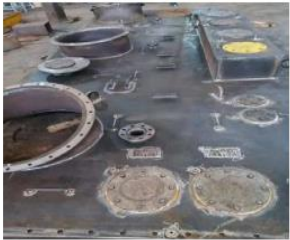
Main transformer Oil tank production
