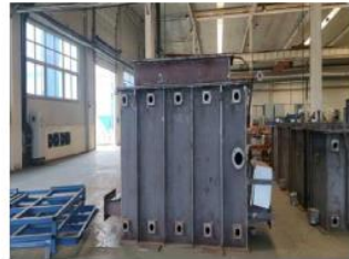
Inverter station Oil tank production
